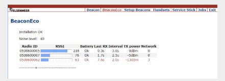
More importantly, you can switch into the ECO Mode, which allows a BEACON ECO to run for typically 10 years with only one set of batteries. In ECO mode you can also change the transmission interval and the network ID.
