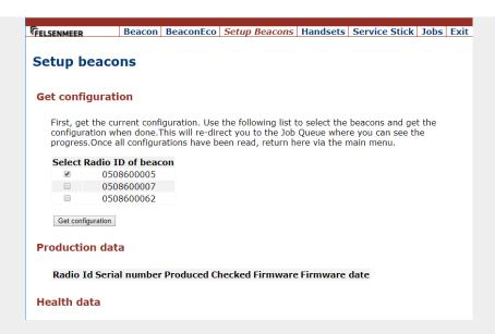
BEACON ECO and CIPOLLINO BEACON, however, can be configured using this product. You have better control over transmission power, compared to using the key. You can also configure a site ID, which is used to distinguish neighboring installations.
